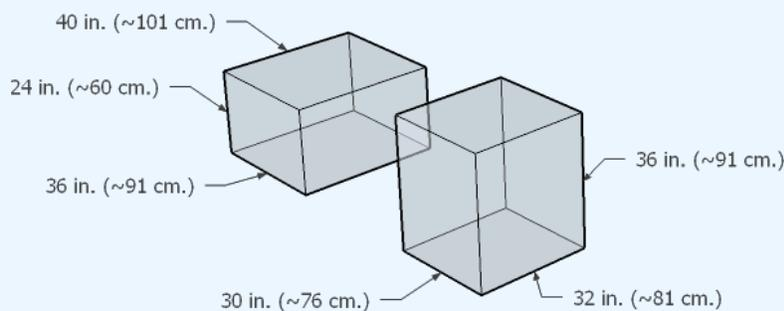
These measurements are intended to be made as if the ROBOT is resting on a flat floor, not relative to the height of the ROBOT from the FIELD carpet.
