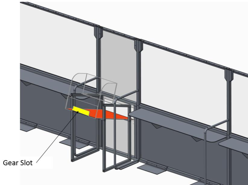
An Overflow LOADING STATION is used to feed FUEL from the OVERFLOW BIN on to the FIELD. Each Overflow LOADING STATION includes a 6 ft. 6 in. (~198 cm) in. tall and 2 ft. 6 in. (~76 cm) wide polycarbonate panel with an opening, aluminum frame, and shelf with backboard. The opening is 2½ in. (~6 cm) from each edge of the loading station, 2 ft. 1 in. (~64 cm) wide, 7½ in. tall (~19 cm), and 2 ft. 1 in. (~64 cm) above the carpet.
