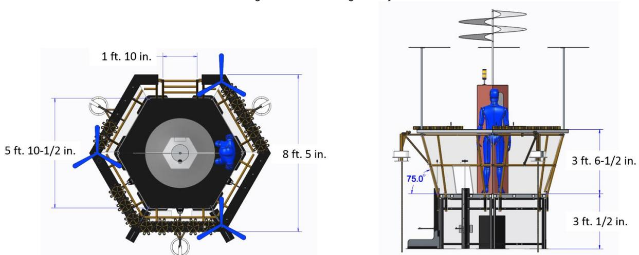
The deck is accessed by a step ladder. The step ladder is 1 ft. 10 in. (~56 cm) wide. Before MATCH play, it is rotated upward and latched to the rail.
