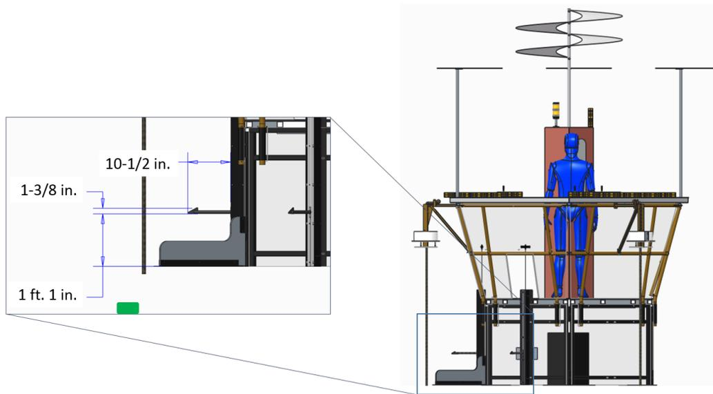
The center LIFT is flanked by two ½-in. (nominal) thick HDPE barriers that radiate out from the adjacent AIRSHIP corners. Barriers are 6¼ in. (~16 cm) tall and extend 2 ft. ¾ in. (~63 cm) out from the leg of the AIRSHIP.
