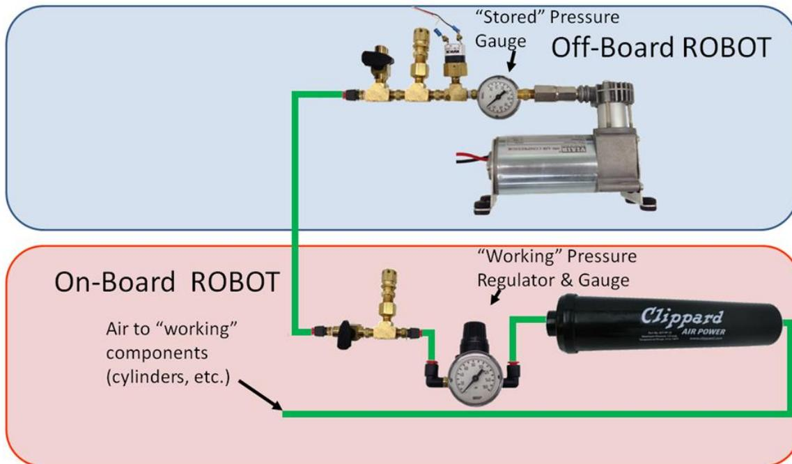
**R92.** The relief valve must be attached directly to the compressor or attached by legal hard fittings (e.g. brass, nylon, etc.) connected to the compressor output port. If using an off-board compressor, an additional relief valve must be included on the ROBOT.
