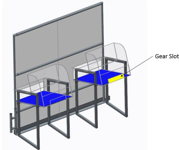
A Return LOADING STATION is used to feed FUEL and GEARS on to the FIELD. Each Return LOADING STATION includes a 6 ft. 6 in. (~198 cm) in. tall and 6 ft. 3½ in. (~192 cm) wide polycarbonate panel with two (2) openings, aluminum frame, and shelves with backboards. The openings are side by side, 1⅜ in. (~3 cm) from each edge of the loading station, 2 ft. (~61 cm) wide, 7½ in. tall (~19 cm), and 2 ft. 1 in. (~64 cm) above the carpet.
