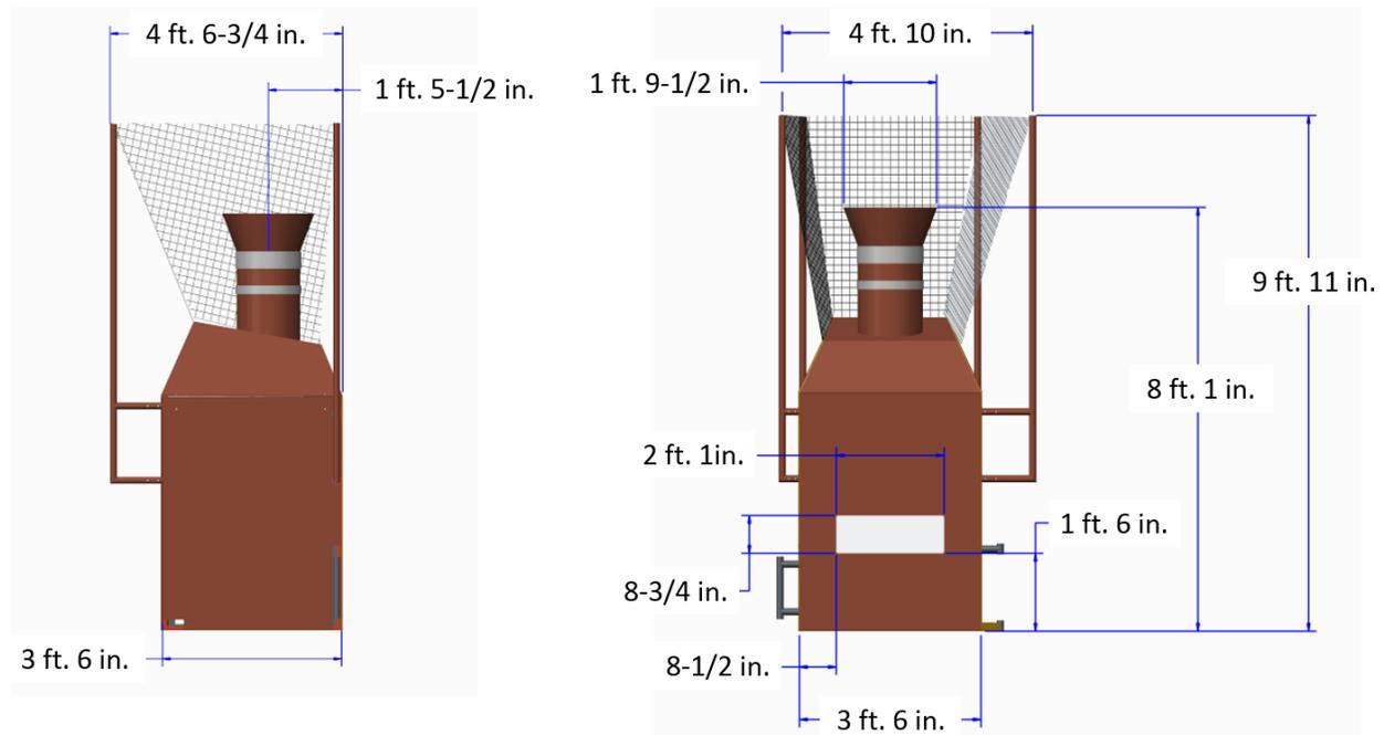
The capacity of the Low Efficiency GOAL is seventy (70) FUEL. The capacity of the High Efficiency GOAL is one-hundred and fifty (150) FUEL. FUEL that exceeds GOAL capacities will fall back on to the FIELD.
