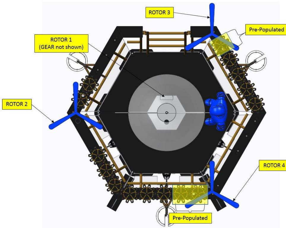
A GEAR set is a series of meshed GEARS that correspond to a specific ROTOR. GEAR sets are installed on AXLES mounted to the rail. An AXLE is a  $\frac{7}{8}$ -in. diameter (~2 cm), 2-in. (~5 cm) long shaft which fits the central hub of a GEAR. The number of AXLES for each GEAR set depends on the ROTOR. Some AXLES are prepopulated with GEARS and indicated in Table 3-1. The number of pre-populated GEARS may change for District Championships or the *FIRST* Championship.
