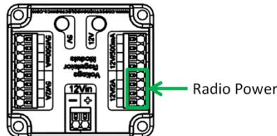
Note that this wiring is different from the wiring for the radio used in 2015, but is identical to the wiring from 2016. When using a 2015 VRM with the OM5P-AN or OM5P-AC radio, the radio should be connected as described above, not to the terminals labeled “Radio”.
