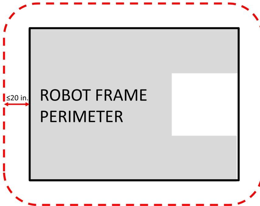
Figure 3-6: FRAME PERIMETER Extension
