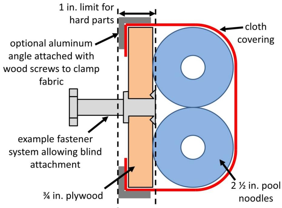
Figure 4-8: BUMPER Vertical Cross Section
