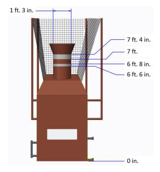
Figure 3-36: BOILER vision target measurements
