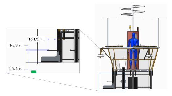
The center LIFT is flanked by two  $\frac{1}{2}$ -in. (nominal) thick HDPE barriers that radiate out from the adjacent AIRSHIP corners. Barriers are  $6\frac{1}{4}$  in. ( $\sim$ 16 cm) tall and extend 2 ft.  $\frac{3}{4}$  in. ( $\sim$ 63 cm) out from the leg of the AIRSHIP.
