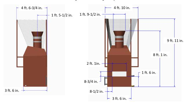
Figure 3-31: BOILER geometry
