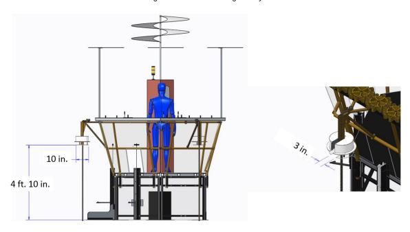
Figure 3-19: TOUCHPAD geometry
