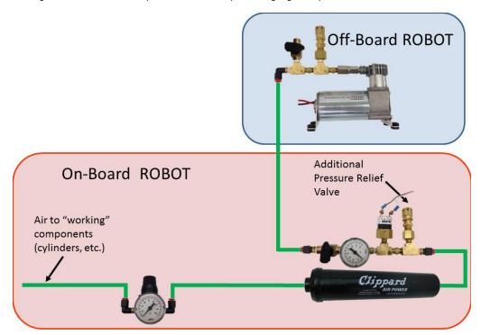
R91. If the stored pressure gauge is kept off-board the ROBOT with the compressor, then only low-pressure (60 psi (~413 kPa) or less) "working" air can be stored on the ROBOT. The "working" pressure gauge must be installed on-board the ROBOT at all times (Figure 8-15).
