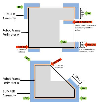
Figure 8-2: BUMPER around full side/corner.
