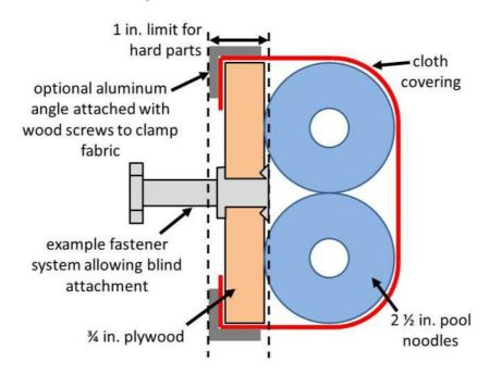
**R30.** Corner joints between BUMPERS must be filled with pool noodle material. Examples of implementation are shown in Figure 8-6.
