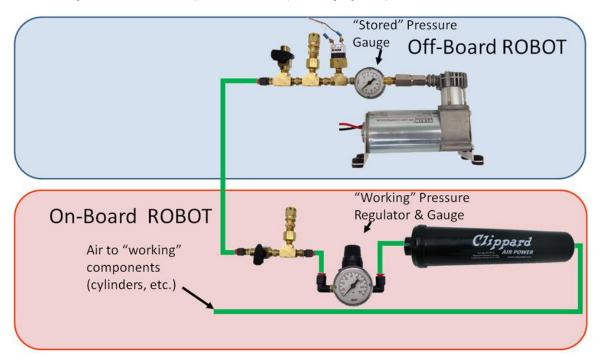
R92. The relief valve must be attached directly to the compressor or attached by legal hard fittings (e.g. brass, nylon, etc.) connected to the compressor output port. If using an off-board compressor, an additional relief valve must be included on the ROBOT.
