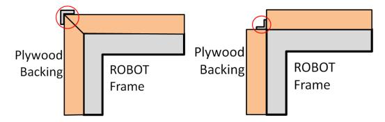
**G.** must attach to the FRAME PERIMETER of the ROBOT with a rigid fastening system to form a tight, robust connection to the main structure/frame (e.g. not attached with hook-and-loop, tape, or tie-wraps). The attachment system must be designed to withstand vigorous game play. All removable fasteners (e.g. bolts, locking pins, pippins, etc.) will be considered part of the BUMPERS.
