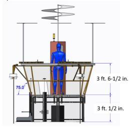
The deck is accessed by a step ladder. The step ladder is 1 ft. 10 in. (~56 cm) wide. Before MATCH play, it is rotated upward and latched to the rail.
