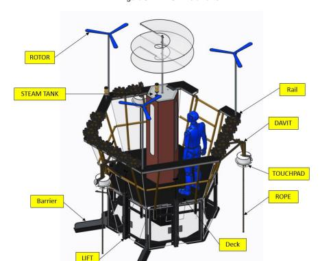
Figure 3-7: AIRSHIP elements
