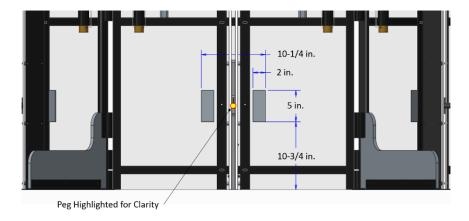
Figure 3-37: LIFT peg vision target dimensions
