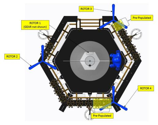
A GEAR set is a series of meshed GEARS that correspond to a specific ROTOR. GEAR sets are installed on AXLES mounted to the rail. An AXLE is a %-in. diameter (~2 cm), 2-in. (~5 cm) long shaft which fits the central hub of a GEAR. The number of AXLES for each GEAR set depends on the ROTOR. Some AXLES are prepopulated with GEARS and indicated in Table 3-1. The number of pre-populated GEARS may change for District Championships or the *FIRST* Championship.
