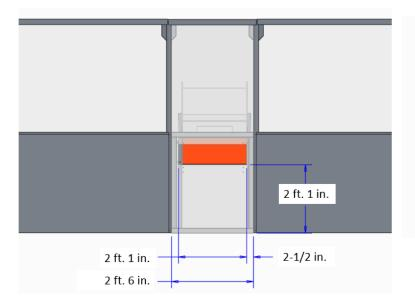
Figure 3-28: Overflow LOADING STATION geometry
