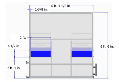
Figure 3-30: Return LOADING STATION geometry
