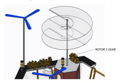
Figure 3-13: GEAR placement to start ROTOR 1
